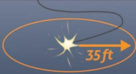
Downed power lines can energize the ground up to **35 feet away**. Even more in wet conditions.
